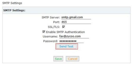
Click the button "Send Test" after configuration and enter the Email address on the following diagram.
